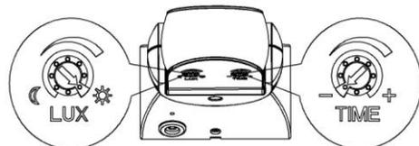
the maximum (sun); turn the TIME knob anti-clockwise on the minimum (-).
