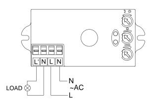
Connect N, L with power; Connect N, L' with load.
