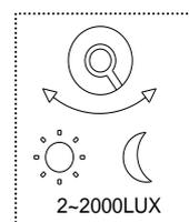
The chosen light response threshold can be infinitely from approx. 2-2000lux. Turn it fully anti-clockwise to select dusk- to-dawn operation at about 2 Lux. Turn it fully clockwise to select daylight operation at about 2000lux. The knob must be turned fully clockwise when adjusting the detection zone and performing the walk test in daylight.
