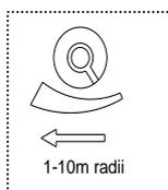
Reach is the term used to describe the radius of the circular detection zone produced on the ground. After mounting the sensor light at a height of 2.5m, turn the reach control completely in anti-clockwise direction to select minimum reach (approx. 1 m radius), and turn the reach control completely in a clockwise direction to select the maximum reach (approx. 10m radius).
